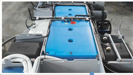
Optimum axle load is given as the weight of the installations is distributed across the double floor just so; the two large water tanks, for example, are located in the centre of the rear axle.
