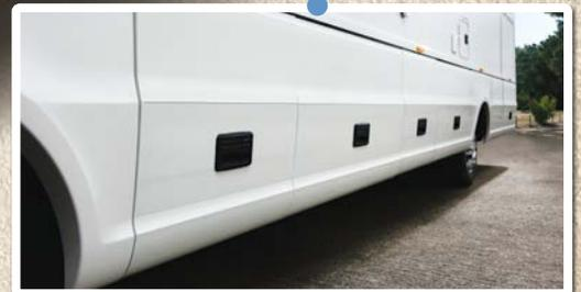
The elaborate side skirts made of varnished aluminium profiles give the Flair a sporty look on the outside. They cover the chassis frame and the retracted outside step.
