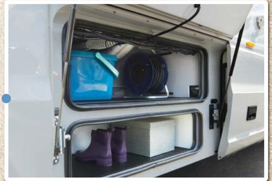
All installations and storage areas in the double floor can be accessed conveniently and in a way that's conducive to service – via the fully insulated bus flaps.
