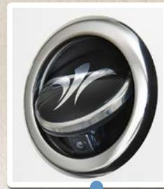
The rear is topped off by LED tail lights with the unique, threefold night signature and the perfectly integrated, dirt-proof rear-view camera (optional) set behind the logo.
