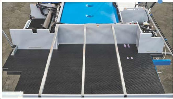
The combination of subfloor and floor panel ensure high rigidity of the chassis and, as a result, excellent driving qualities. What's more, the insulation afforded by the double-sided aluminium sandwich minimises road noise in the box construction.
