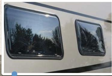
The optional double-glazed side windows ensure better insulation and also offer up to 80% more heat protection than conventional, single-glazed side windows.
