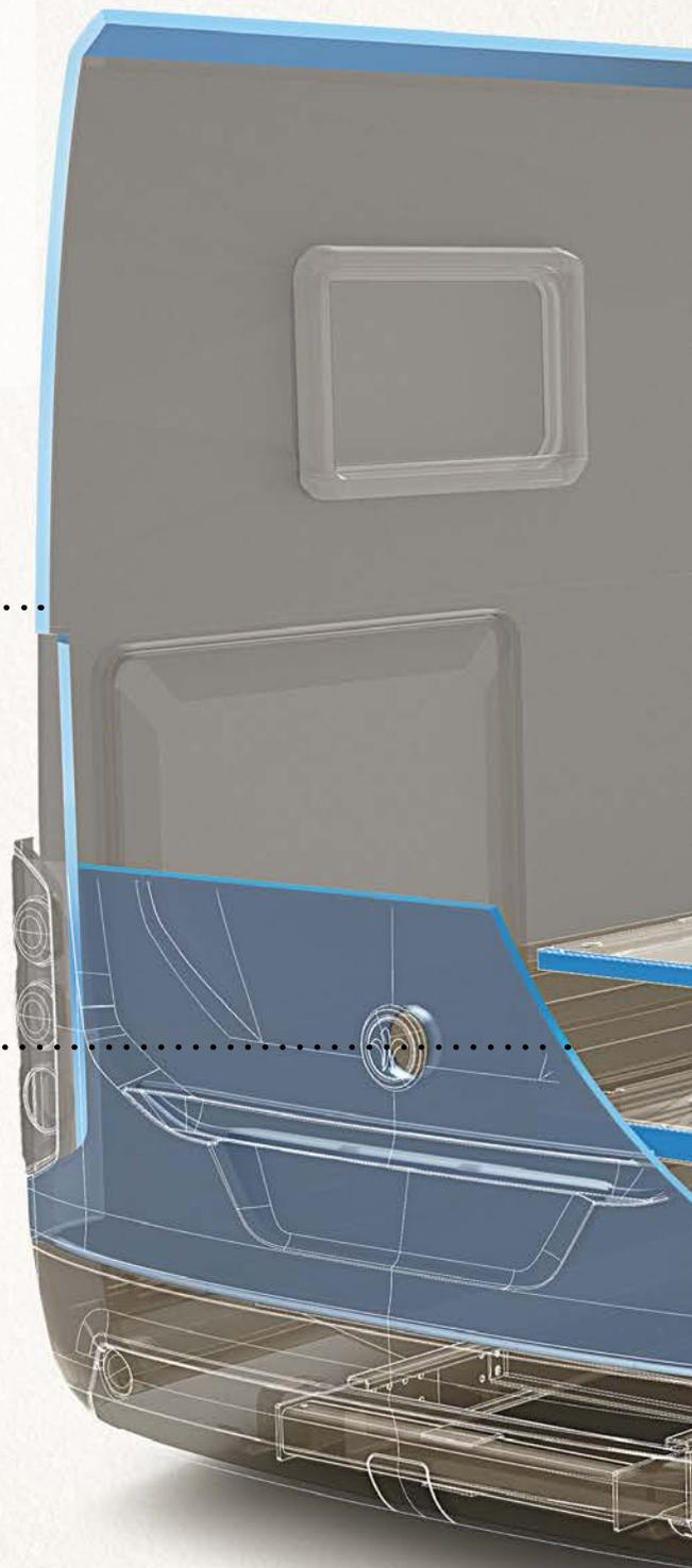
The connection between the roof and the side walls is also free of cold bridges thanks to double-sided aluminium.
