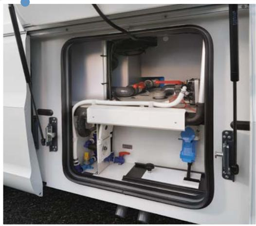
The service flap is located on the left side, making it easier to pull up at service stations. This also prevents smells or staining from occurring on the sunny side of your motorhome.
