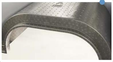
The rear wheel casings are insulated with expanded polypropylene to absorb sounds and the cold in an outstanding manner.
