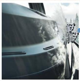
The rear ventilation on the windscreen works in conjunction with the convective heaters like a thermal screen.
