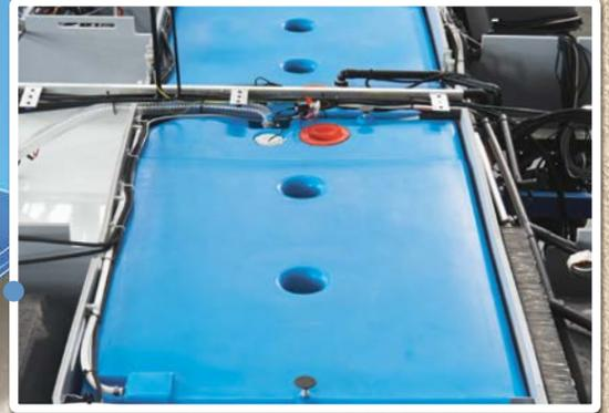
The large water tanks are mounted in the heated double floor insulated with a double-sided aluminium sandwich and so won't freeze at sub-zero temperatures. The water tanks can be removed and replaced via the rear garage.
