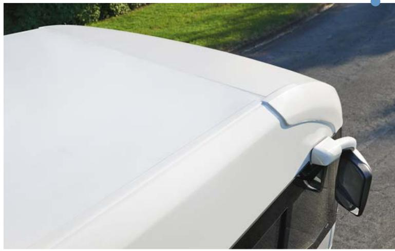
The flush-mounted transition from the front mask to the roof prevents back-pressure of water and ensures that the water runs off to the front.
