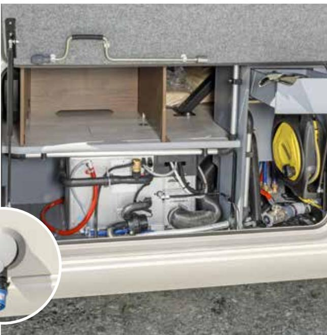
Self-retracting cable reel with 15 m of cable and central supply system
